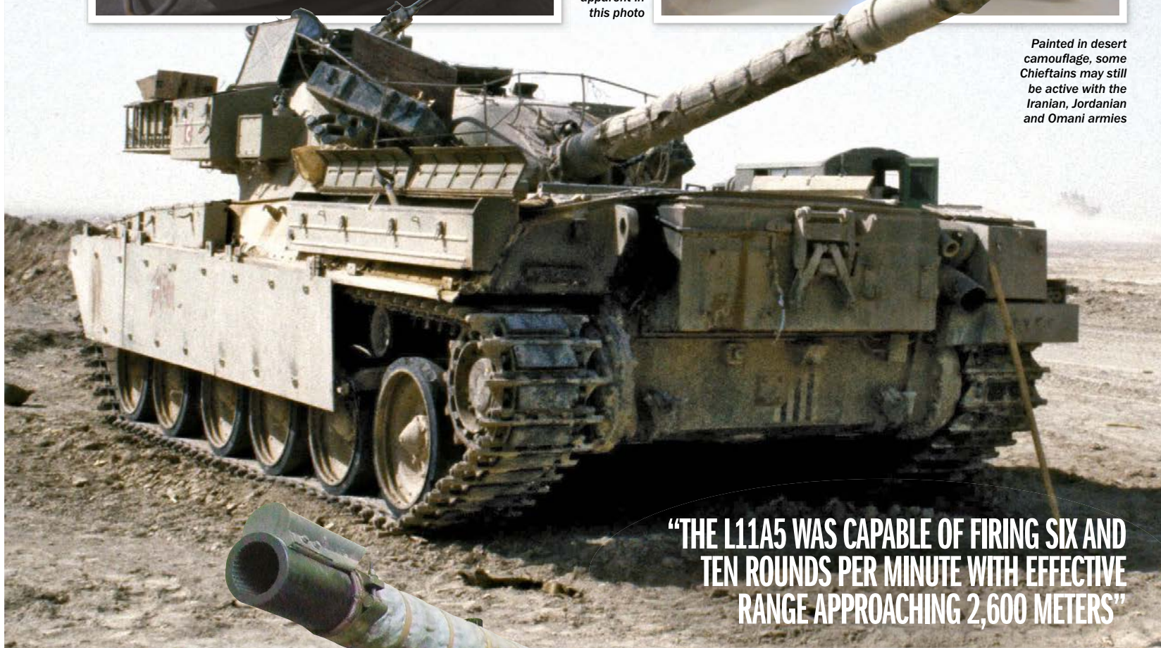
Right: Secondary smoke grenade launchers are visible on either side of the turret. Note the cupola-mounted 7.62mm L37A1 machine gun
